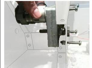
4 Screws holding elevation motor onto Davit Center along with the small white spacers
