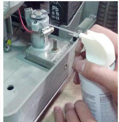
**Try to start the machine after following this cleaning process, if the problem persists then further inspection of the sweep sensors is required. Proceed to the next step of removing the Platform.**
