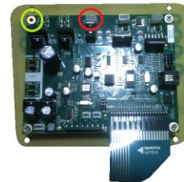
Feed motor plug circled red
